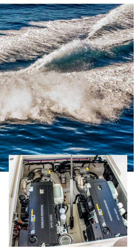
**TOP** Flat-out speed is a shade over 30 knots. **ABOVE** The twin 370hp Volvo Pentas are happy mates for the 395's sporty hull.
